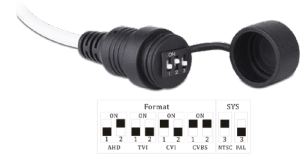
DIP Switch for Output Selection
